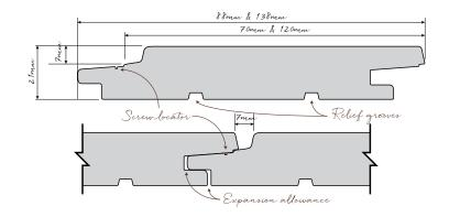
• Allowances have been made for expansion gaps, but must be implemented using a 6mm spacer to achieve a uniformed shadow line.
