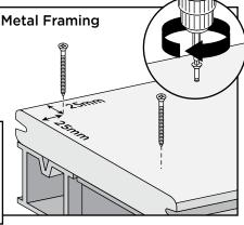
For wood framing, and if using Trex Universal Hidden Fasteners, pre-drill and toenail an approved screw at an angle in groove at both ends 25mm from board end and center of each board.
