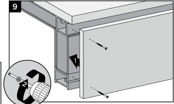
**NOTE:** Fascia wider than 184 mm will require more detailed fastener requirements. Fascia boards are not allowed to carry loads from decking. Contact a Trex representative for more detail.
