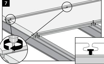
Installing Last Deck Board (Square-Edge Board Recommended)
