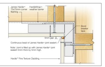
FIGURE 26 SEALANT FILL OPTION - CAVITY TRIM
