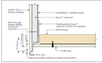
FIGURE 20 FACADE/SOFFIT JUNCTION
